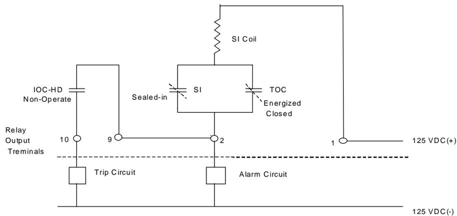
Figure 1 IAC66K Relay Internal Configuration
